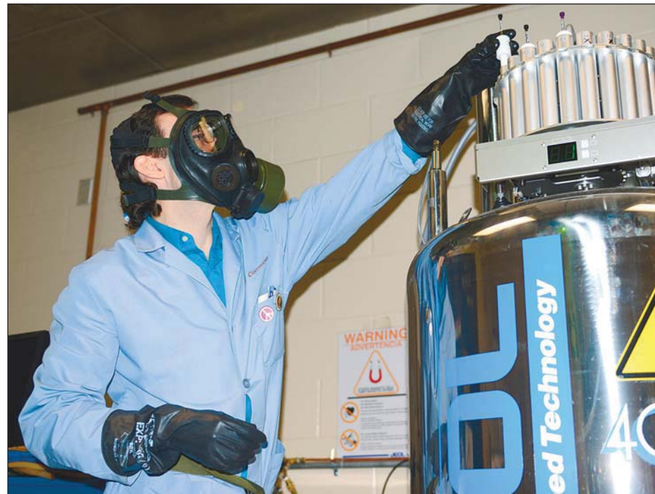
Chemist David McGarvey, Ph.D., of the Army's Edgewood Chemical Biological Center at APG, inserts a swatch of fabric into a nuclear magnetic resonance spectrometer. The swatch of uniform fabric has been treated with chemicals that can break down chemical warfare agents. The spectrometer is used to determine what those chemical warfare agents are broken down into when they come in contact with the fabric treatment.
